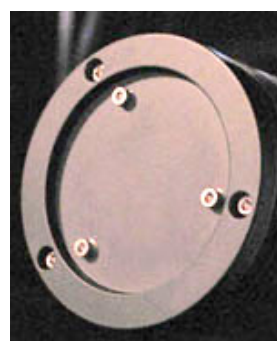
Figure 2. Meade six-screw secondary.
