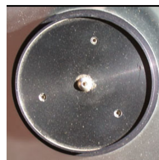
Figure 1. Celestron secondary with set-screws.
