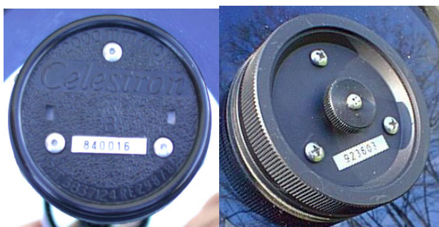
Figure 2. Celestron secondary with three machine screws; non-Fastar on left, Fastar on right.
