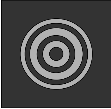
Figure 3. Star pattern of collimated scope.
