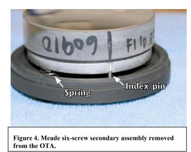
Finally, it's possible for the index pin protruding from the secondary housing (Figure 4) to jam against the secondary mirror mounting plate such that collimation cannot be adjusted.
