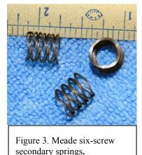
compressed position; see the next paragraph.) Take a look at the secondary mirror reflected in the primary. If it is tilted to the side no matter what you do with the collimation screws, a spring is probably to blame. There's no reason to panic, though; this situation is easily remedied.
