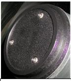
One of the disadvantages to the three-screw design is the limited amount that a collimation screw could be turned before it became tight or loose. This amount was often less than one-half turn, so collimating became an exercise in manipulating all three screws until the secondary was both collimated and held at the correct tension by the screws. Furthermore, access to the secondary mirror required removal of the corrector plate.
