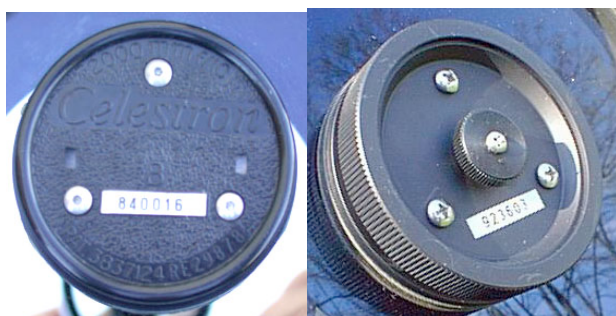
Figure 2. Celestron secondary with three machine screws; non-Faster on left, Faster on right.
