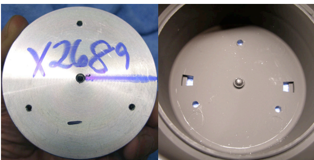
Figure 4. CPC 1100 secondary mirror backing plate (left) and inside of the secondary housing (right).
