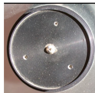
Figure 1. Celestron secondary with set-screws.
