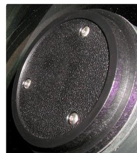
Figure 1. Meade three-screw secondary.
